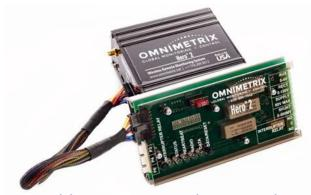
**Rectifier & Test Station Monitors**
