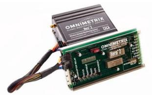
**Rectifier & Test Station Monitors**
